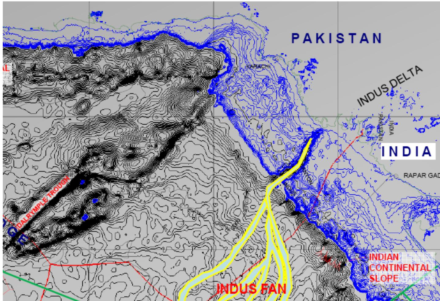
Crossing the Indus Canyon is the main technical impediment to a shallow water coastal route. It is deep, turbulent and can change location. Directional Drilling of multiple lines beneath it may be theoretically possible but remains a high risk solution.
